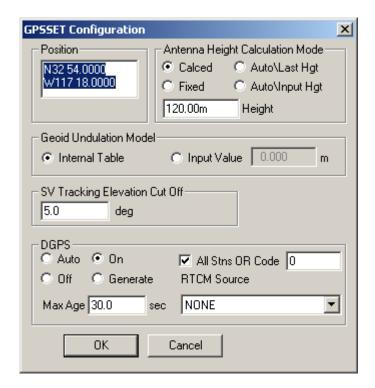
This dialog allows for parameters to be set on the receiver which will be used by the receiver for position calculations.
