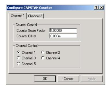
If you determine that the incoming cable count is incorrect, possibly due to a miscalibration of the counter itself, a compensating Scale Factor can be entered here. This can also be used to convert incoming units to the desired units. Also an offset value can be entered in the appropriate field. This value will be added to the result of the Scale factor and the raw cable count.
