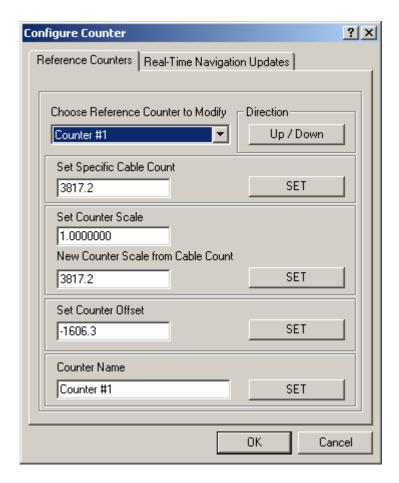
This page is used in conjunction with the Calculations window to maintain up to five reference counts based on the Channel One (cable) count. These reference counts are not used for any real-time calculations and are not logged to any file; they are intended for reference purposes only.
