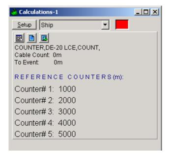
Once the Calculations window has been opened and configured, the five reference counters can be modified using the Reference Counters tab of the Configure Counter dialog. (Note: the Configure Counter dialog can be directly accessed from the Calculations window by clicking the 🔜 icon in the Calculations window.)
