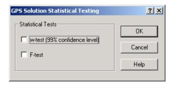
This dialog box provides you with the ability to enable or disable statistical w test and F tests. By default, both of the w-test and the F-test are turned off.
