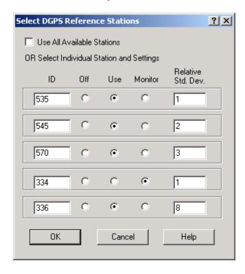
The Select DGPS Reference Stations dialog box allows you to define which reference stations will be used by WinFrog in its Multi-Ref solution. You can either configure WinFrog to simply use all received stations (to a maximum of 5), or you can control the use of corrections, as deemed proper.
