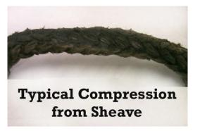
significantly reduced diameter. The fused strands should not be confused with high-tension compression of the rope which might appear similar. With standard urethane coatings, the rope can appear melted after high tension has been applied while the rope is bent around a surface. This is normally not melting and can be worked out with little effort. The rope strength is not affected.
