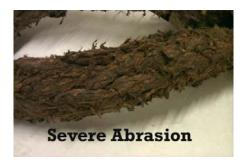
5. Keep a detailed record of the line reference length as well as any damage areas and their approximate locations relative to one or both reference marks. Future inspections should be used to monitor minor damage areas for signs of growth.
