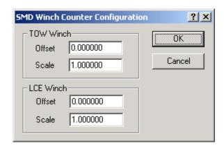
In this dialog box the operator can enter an offset that will be added to the observed tow wire or cable count. A scale factor can also be entered that will be multiplied by the observed tension value to produce a final scaled tow wire or cable tension in Tonnes
