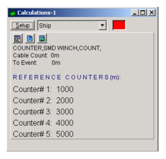
Once the Calculations window has been opened and configured, the five reference counters can be modified using the Reference Counters page of the Configure Counter dialog. (Note: the Configure Counter dialog can be directly accessed from the Calculations window by clicking the configure Counter dialog.)
