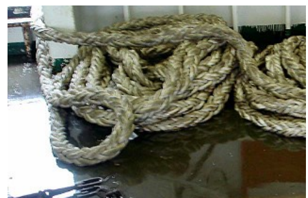
Ropes badly stored on wet deck
