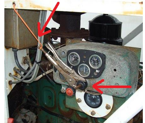
Rigged gear using vise grips and a rubber band.
