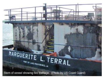
In June 9, 2012, about 1705 central daylight time, the towing vessel *Marguerite L Terral* was pushing 12 empty barges on the Mississippi River near Hickman, Kentucky, when the vessel's port engine caught fire. The six person crew tried unsuccessfully to extinguish the fire before evacuating onto one of the barges. No one was injured and no pollution resulted from the fire. The damage to the vessel was estimated to be \$2.6 million.
