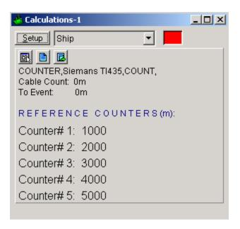
Once the Calculations window has been opened and configured, the five reference counters can be modified using the Reference Counters page of the Configure Counter dialog. (Note: the Configure Counter dialog can be directly accessed from the Calculations window by clicking the licon in the Calculations window.)
