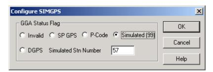
From this dialog you can select the quality of the GPS data to be generated by setting the GGA status flag. If the DGPS option is selected, a simulated reference station ID number can also be entered.
