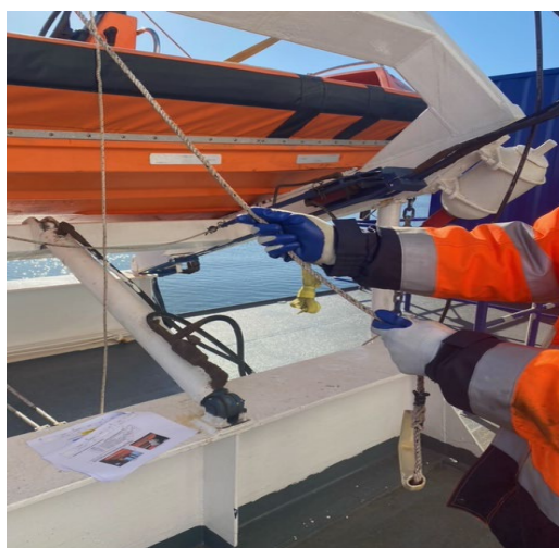
Emergency Lower Line
